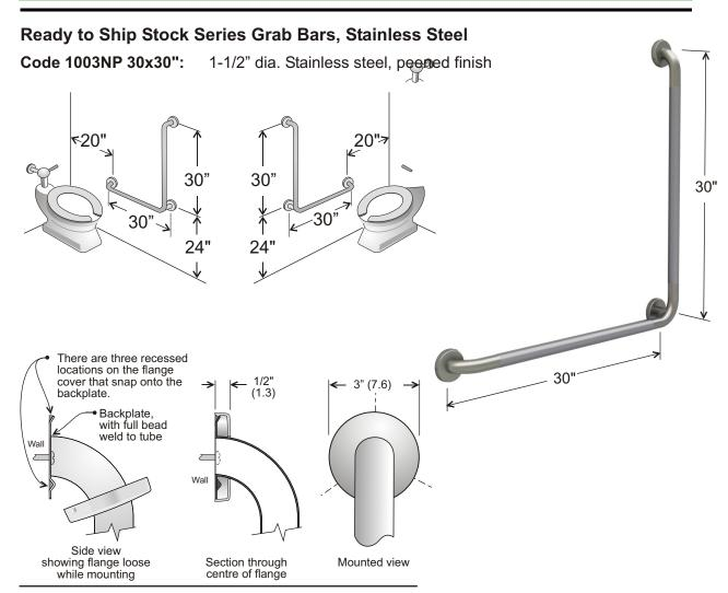
Concealed mounting screws, using snap flange, on "SP & NP" codes
