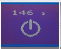
Customizable timeout countdown shuts the machine off after 5 minutes of inactivity for enhanced safety and efficiency.
