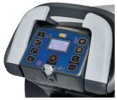
Every facet of the SC500 has been fine-tuned for an optimal user experience. The unique multi-function display and control panel grants managers—using the yellow Superuser key—access to adjustable cleaning parameters. Operators—using the gray key—are able to start cleaning at the beginning of their shift. They don't need to take the time to change machine settings before they start.
