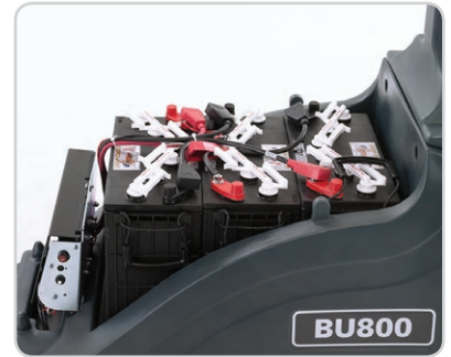
Choose between wet cell or service-free AGM batteries. Onboard charger is standard.
